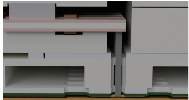
Figure 2. Segmented tri-morph actuator stacks with a connecting conductive crossbar and the plunger connected at the free-moving end.
