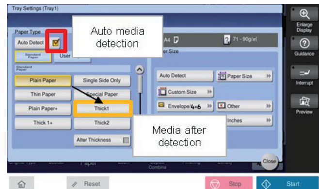
Figure 10. Automatic media detection is enabled by default on the control panel. After detection, the detected paper is automatically displayed. [1]
