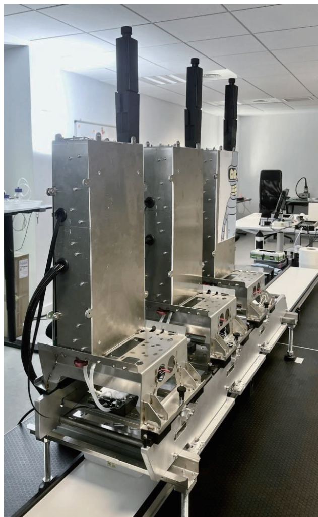
Figure 6. Prototype Print Engine in a 150npi print configuration
