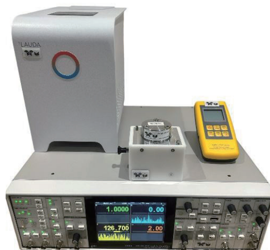
Figure 1. TriPAV equipment with lock-in amplifier, thermostat circulator, digital thermometer.
