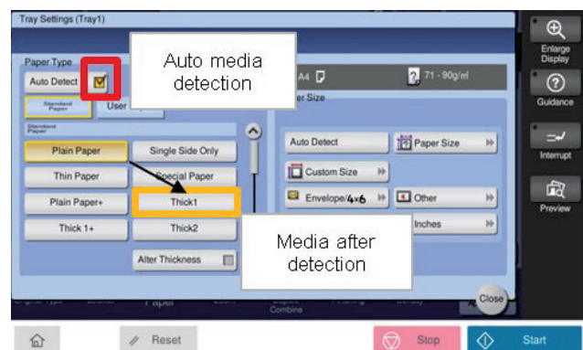
Figure 10. Automatic media detection is enabled by default on the control panel. After detection, the detected paper is automatically displayed. [1]
