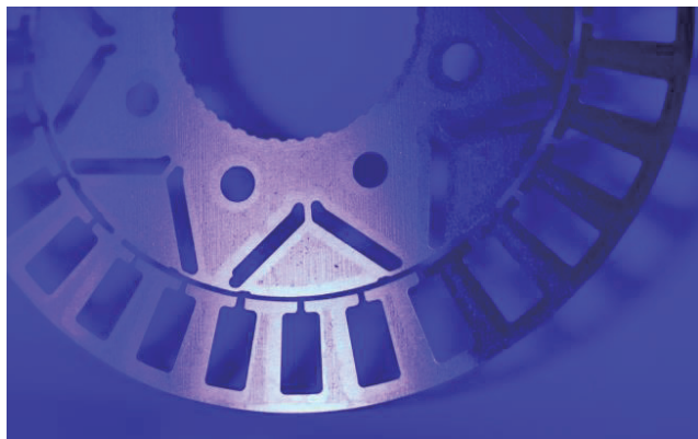
Figure 5. Temperature sensitive adhesive printed on e-motor rotor sample.
