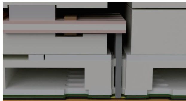
Figure 2. Segmented tri-morph actuator stacks with a connecting conductive crossbar and the plunger connected at the free-moving end.
