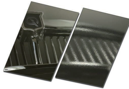
Picture 2. Example of Sharpness/DOI measurement
